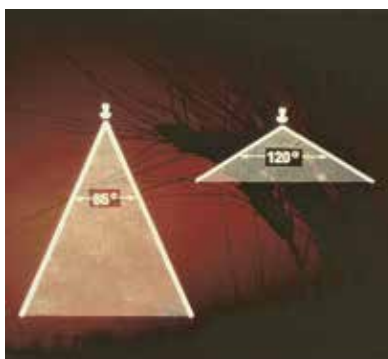
Nozzle spray angles of 65 and 120 degrees.
