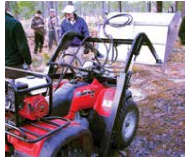
Grass seed harvester on an ATV.
