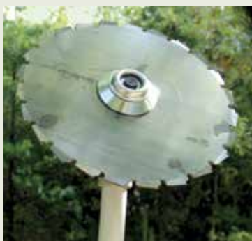
Brushsaw blade with chainsaw-like teeth.
