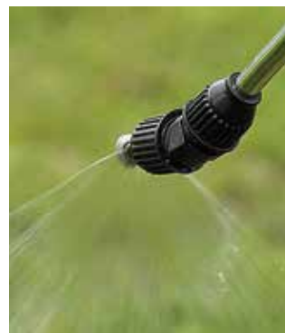
Flooding nozzle spray pattern.
