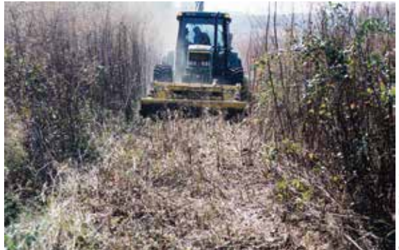
Wetblade brush mower applies herbicide while cutting.
