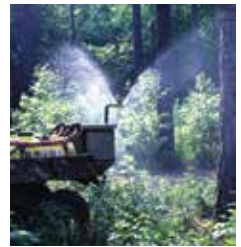
Spray pattern of two Boom Buster nozzles.
