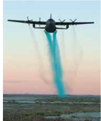
C-130H aircraft and Modular Aerial Spray Systems (MASS).
