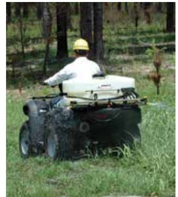
ATV mounted sprayer with a boom.
